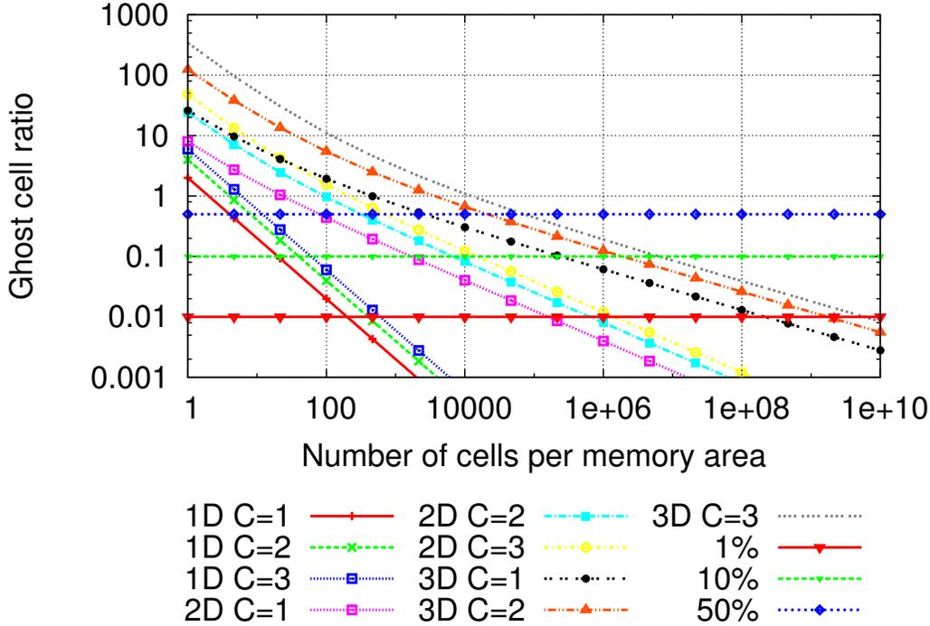
Figure 5: Ghost cell ratio in function of  $n$  for various configurations.
