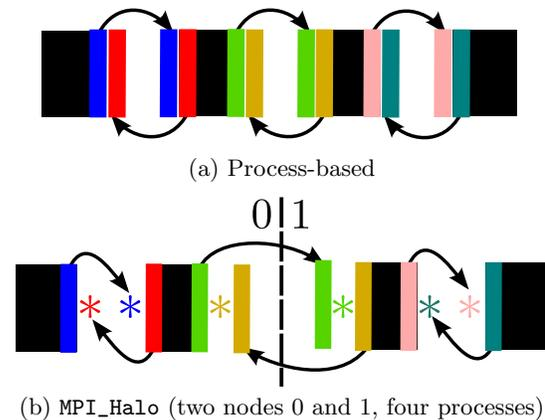
Figure 7: Halo-cell buffer comparison between process-based domain splitting and our node-based MPI\_Halo approach when considering a 1D splitting.
