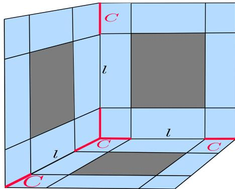
Figure 2: Deriving ghost-cell count from the characteristic length (cube-embedding).
